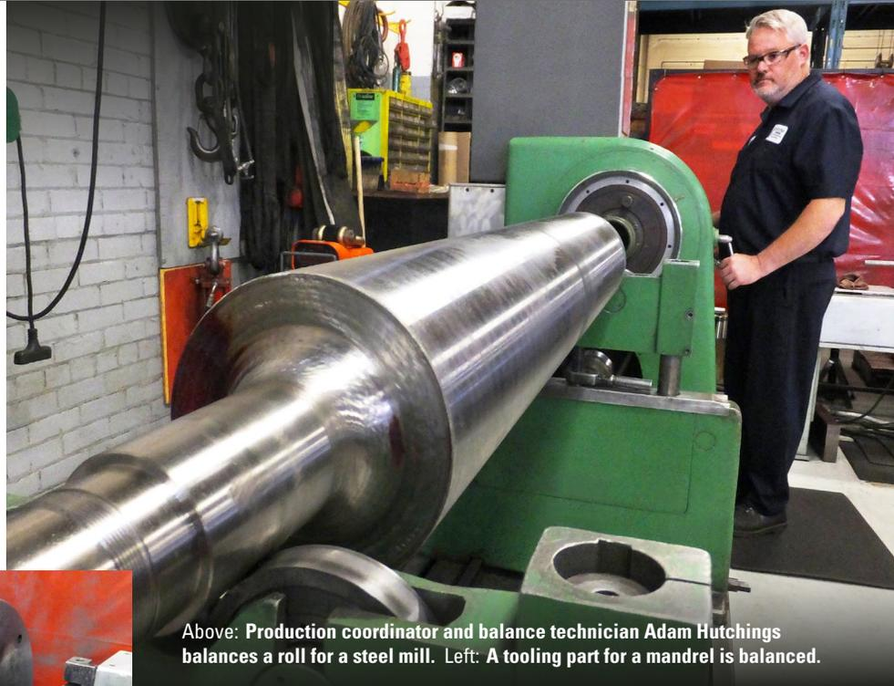
Above: Production coordinator and balance technician Adam Hutchings balances a roll for a steel mill. Left: A tooling part for a mandrel is balanced.
