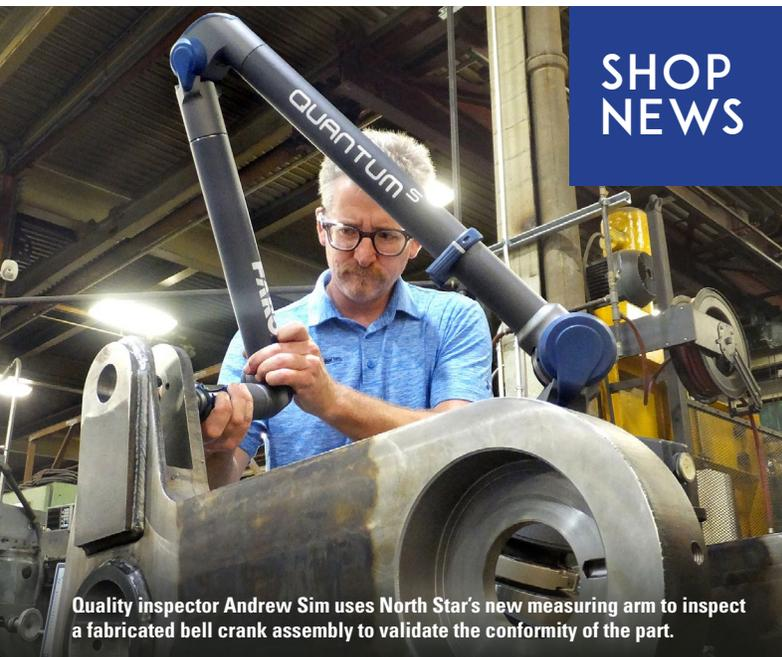
Quality inspector Andrew Sim uses North Star's new measuring arm to inspect a fabricated bell crank assembly to validate the conformity of the part.
