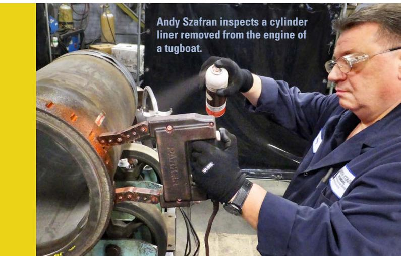
Andy Szafran inspects a cylinder liner removed from the engine of a tugboat.
